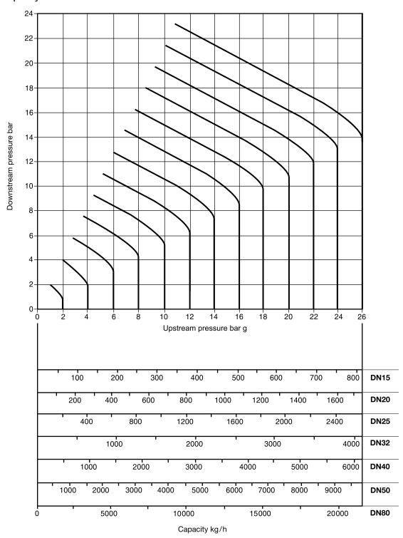
**Note**: The capacities quoted on the above charts are based on valves fitted with external pressure sensing pipes. Reliance on the internal pressure sensing pipe will mean that capacities may be reduced. In the case of low downstream pressure this reduction could be up to 30% of the valve capacity.
