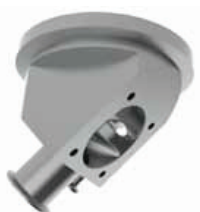
Tank bottom valve weld installation at low point of vessel base enabling optimum drainage, cleaning and sterilization
