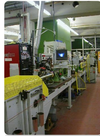
Metal Bellows Production - Tube welding
